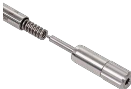
Fig. 8 Insert the spring/punch assembly inside the handle and screw the adjustment knob.
