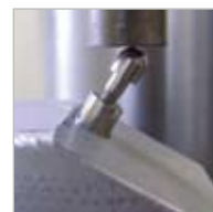
Mechanical testing of fatigue life. Test machine (high frequency).
